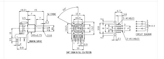
Single unit with R.G.B LED & push on switch -0.5sw RD12S1FV1
