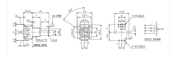
Single unit with R.G.B LED & push on switch -0.5sw horizontal type RD12S1FH1
